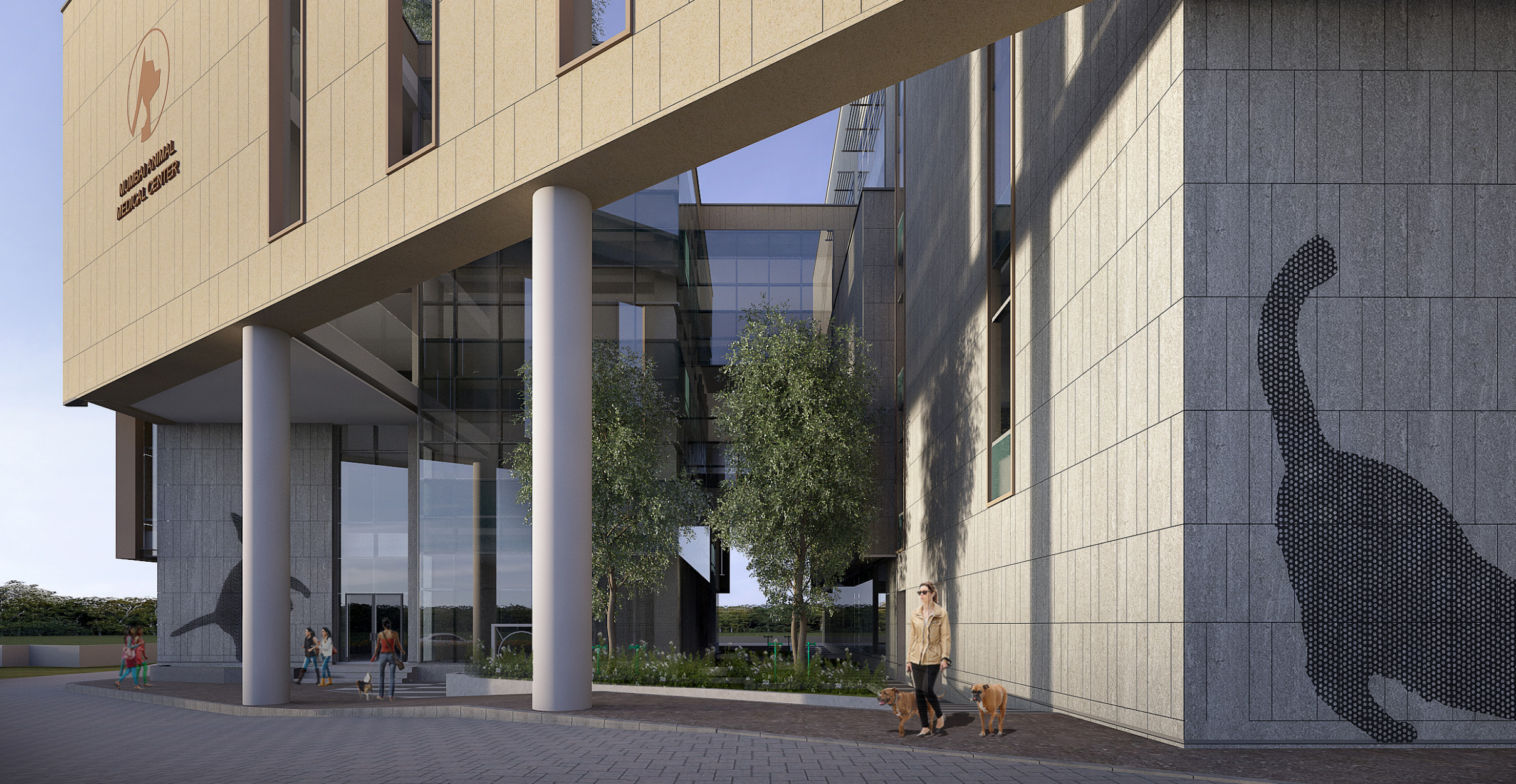
The lower two floors have been made to appear lighter by using structural glazing on the external facade. The public areas and exam rooms are connected with the outdoors visually by creating this transparent screen. The solid granite clad envelope runs around the building volume on all sides and appears to be a floating element that binds the whole mass.
