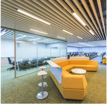
The entire office is on a raised access floor finished with bright, staggered carpet. The spine has rafter ceiling which, visually pierce into the enclosed spaces making the spine corridors look wider. The open office have modular ceiling with linear light fixtures integrated within the ceiling.
